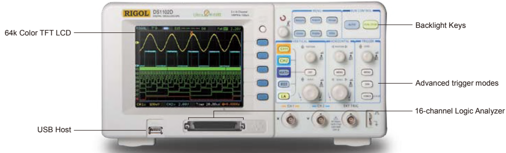
Product Dimensions: Width×Height×Depth=303mm×154mm×133mm Weight: 2.4 kg
